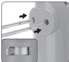
**NOTE:** While using kneaders; There are single and double rims on kneaders. Place the kneader with single rim in the slot on the right (R) side of the product. Place the kneader with double rims in the slot on the left (L) side. Otherwise the dough mixture move to the product main body.
